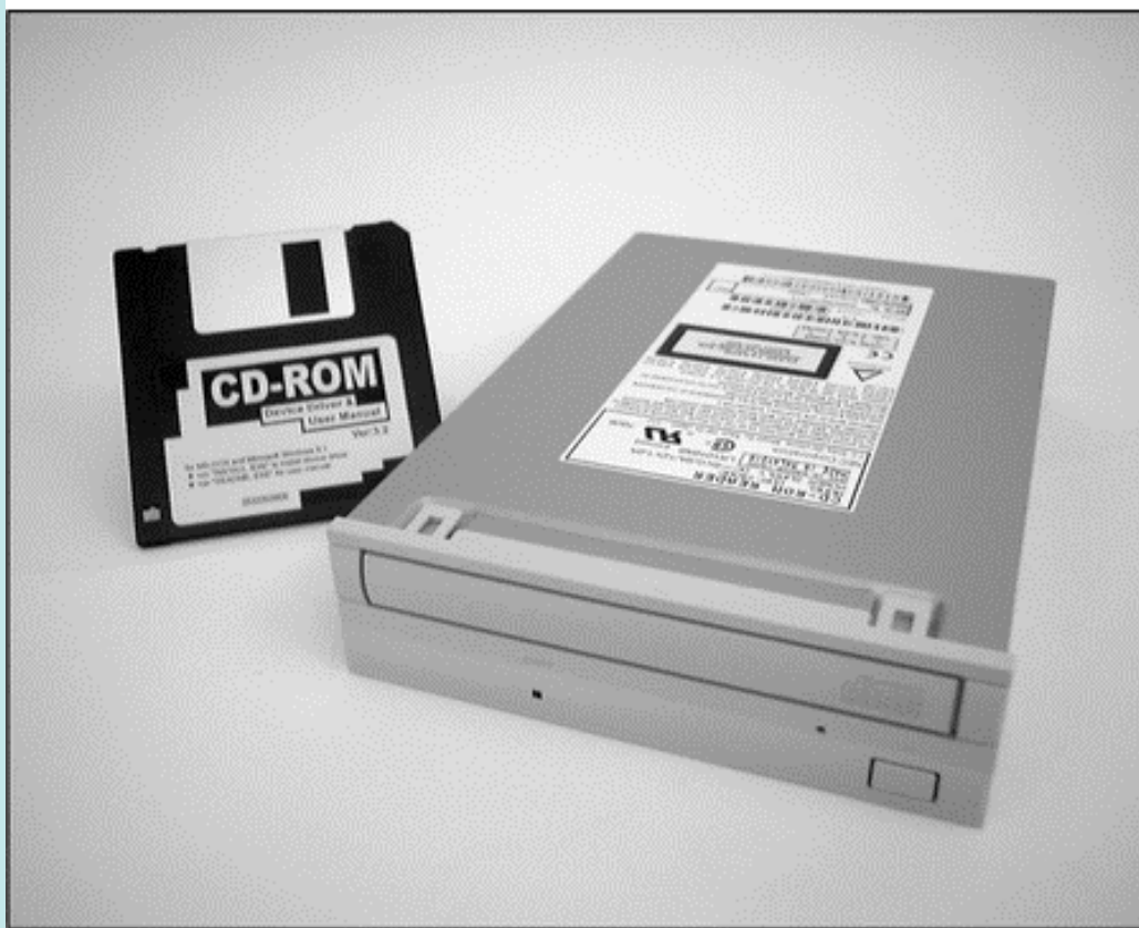
Figure 2-18 A device such as this CD-ROM drive comes packaged with its device drivers stored on a floppy disk or other media. Alternately, you can use device drivers built into the OS.
