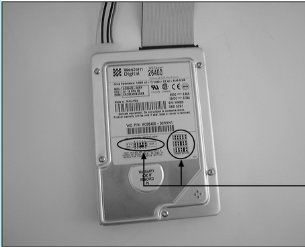
Figure 8-12 An IDE drive most likely will have diagrams of jumper settings for master and slave options printed on the drive housing
