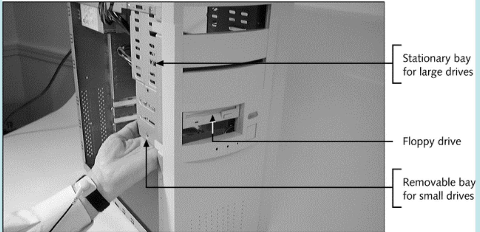
Figure 8-14 Line up the floppy drive in the removable bay so it's flush with the front of the case
