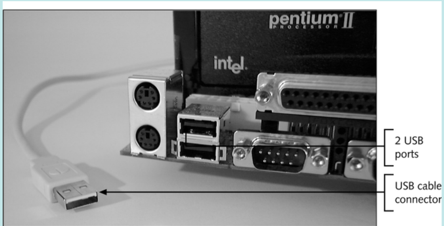
Figure 10-9 A motherboard with two USB ports and a USB cable; note the rectangular shape of the connection as compared to the nearby serial and parallel D-shaped ports
